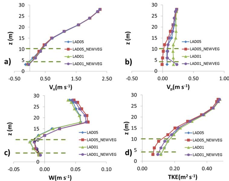
**Figure 3.** Vertical profiles of average flow properties over the study street. a) wind speed normal to street ( $V_n$ ); b) wind speed parallel to street ( $V_p$ ); c) vertical wind speed ( $W$ ); and d) turbulent kinetic energy (TKE). Dashed lines indicate new trees location.
